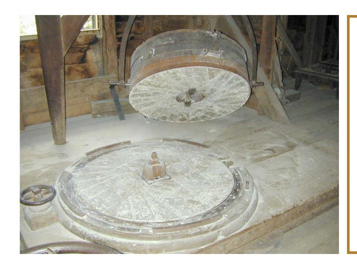
The crane mounted above the millstones allows the upper "runner" stone to be lifted off. The stones can then dressed. The runner stone weighs about 1,500 pounds.
