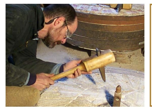
The proper technique for using the millpick is to lift it with the left hand and guide its fall with the right. You never use your wrist to lift the pick, the wrist only guides the picks fall. The force of the picks blow on the stone is determined by how high the left hand lifts the pick.
