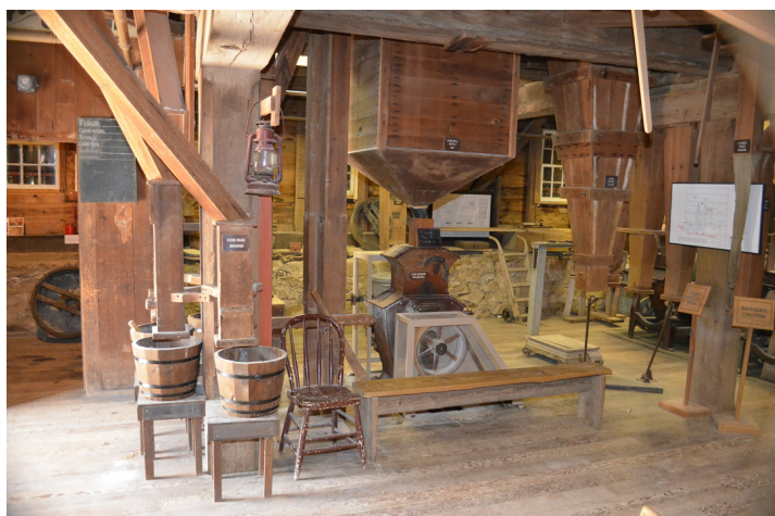
The corn milling plant. The bagging chutes are on the right.
