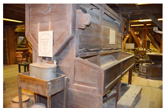
The “Big Bolter” sifted the flour from the millstones into three different grades.
