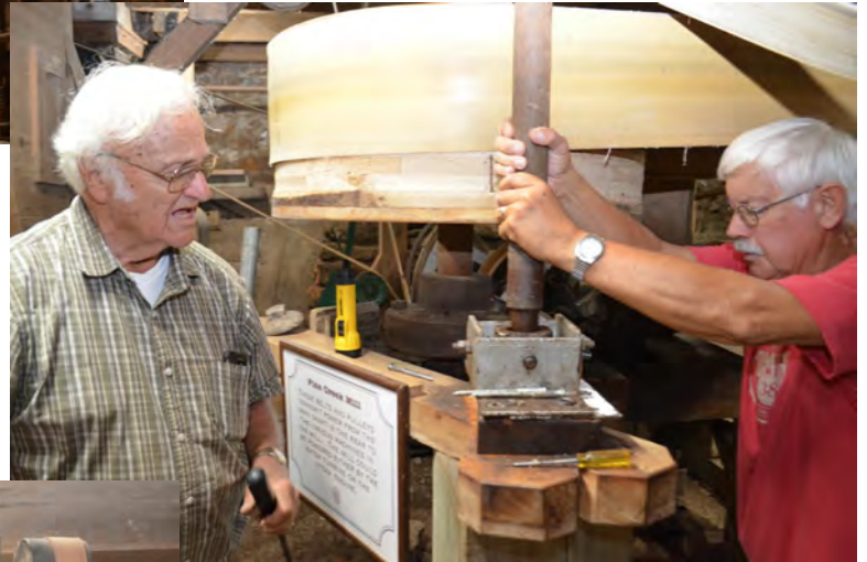
At right Clarence Klauer and Dick Stoltenburg are adjusting the thrust bearing for the smutter's drive pulley shaft.
