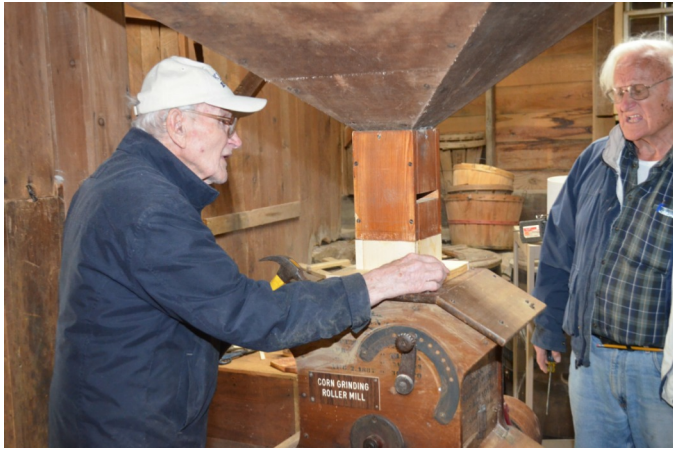
The Klauer brothers Dick and Clarence are working on restoring the in-feed on the corn mill. The old mouse eaten rubber connection has been replaced.
