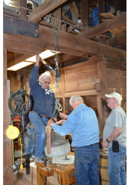
Dan Litwiler (on the right) is being shown how to use the hoisting fixture to lift the runner stone off of the mini-mill.
