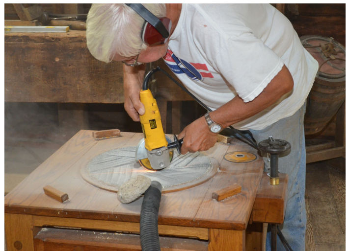
Above Dick Stoltenburg is dressing the mini-mill's bed stone. He is using a special stone cutting blade in the angle grinder.
