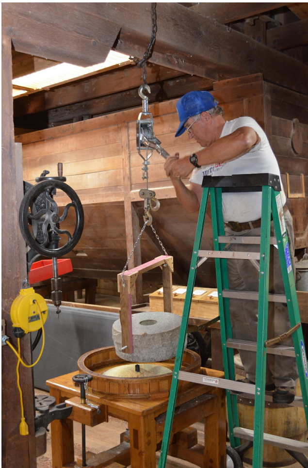
At left Hank Mann testing the new runner stone lifting frame that we built.
