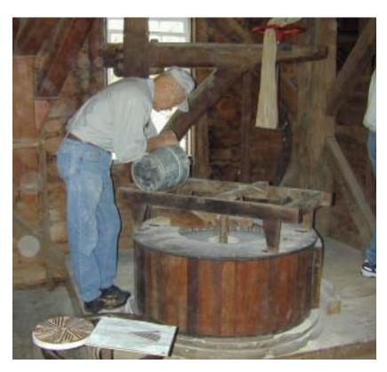
Pine Creek Mill third plant consists of a set of 36" French millstones. These were used to grind Buckwheat and Rye. Buckwheat is not a wheat at all. Its a member of the Rhubarb family and is used only for making pancakes. The black triangular shaped seeds make a grayish pink flour.
