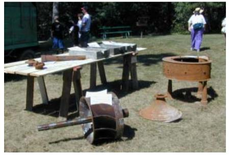
At the left you can see the restored turbine rotor. Extensive work had to be done to restore the worn blades. A new shaft was manufactured and the original Lignum Vitae wood thrust bearing replaced with UHD plastic.
