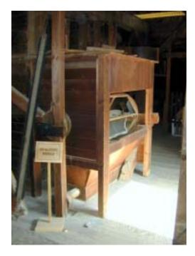
Above is what we think is one of the original 1848 bolters. The construction is quite different from the other machines and appears to date from a earlier period. The bolter is used in the corn milling plant to sift (bolt) corn meal from raw ground corn. Originally the hexagonal rotating reel was covered with silk cloth for bolting flour. For corn meal it was covered with fine metal screen wire. This machine will be restored in 2003.
