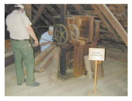
At left are the heads of just three of the many bucket elevators in the mill. From the elevators a complex system of chutes (trunks) lead to various bins and machines. By setting the gates in the chutes the flow chart of the mill could be changed as suited the milling work to be done.
