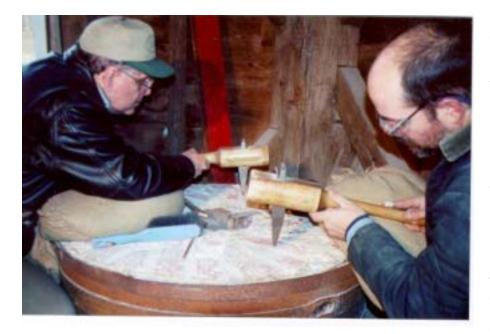
At a busy mill the stones would have to be sharpened at least once a week. The surface of the stone would have to be trued up using paint and straight edge much as a machinist would use bluing.
