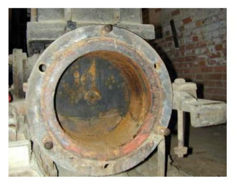
This photo shows the interior of the steam engine cylinder and the piston. The cylinder was about 1/4 filled with fine sand when we removed the head. The head is retained by three bolts and three studs. The head gasket was completely gone. It took a four foot "helper" bar on the wrench to break the nuts free. When opened we found the cylinder partly filled with sand from the frequent flooding the mill endured during the spring thaws.
