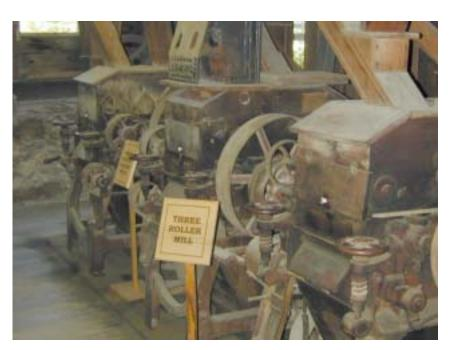
The three flour milling roller mills. Each machine has two separate mills in it. They are driven by a line shaft in the basement below them.
