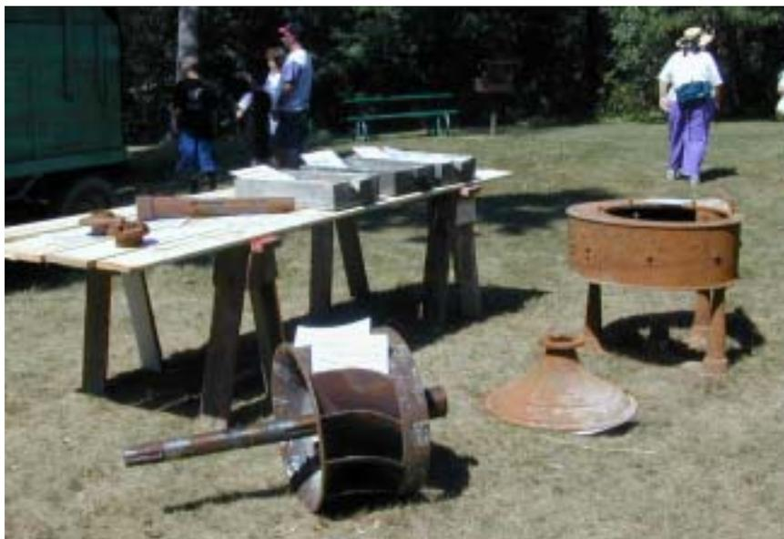
At the left you can see the restored turbine rotor. Extensive work had to be done to restore the worn blades. A new shaft was manufactured and the original Lignum Vitae wood thrust bearing replaced with UHD plastic.
