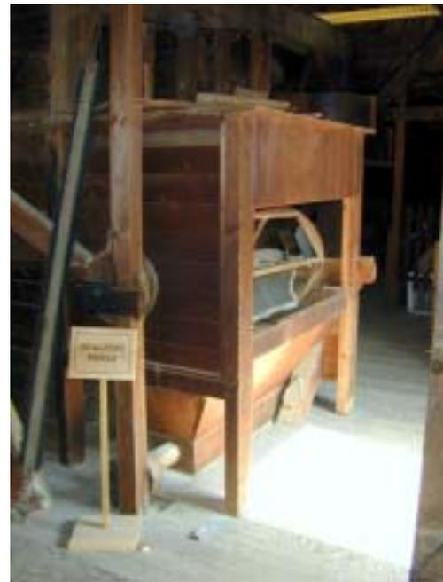
Above is what we think is one of the original 1848 bolters. The construction is quite different from the other machines and appears to date from an earlier period. The bolter is used in the corn milling plant to sift (bolt) corn meal from raw ground corn. Originally the hexagonal rotating reel was covered with silk cloth for bolting flour. For corn meal it was covered with fine metal screen wire. This machine will be restored in 2003.
