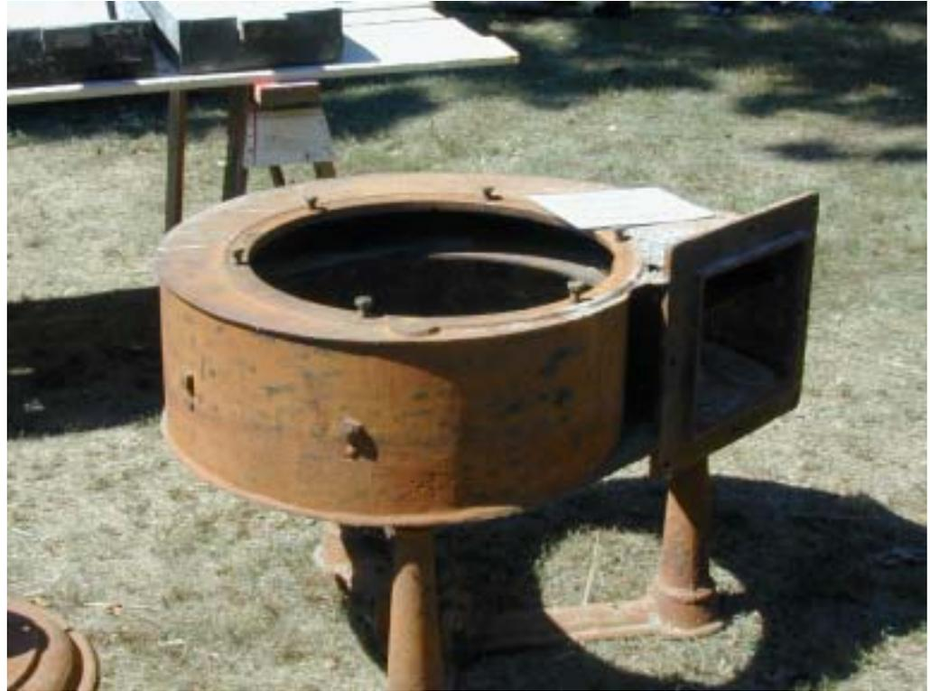
With the original dam the turbine had a head that could generate 20 HP at 220 RPM.
