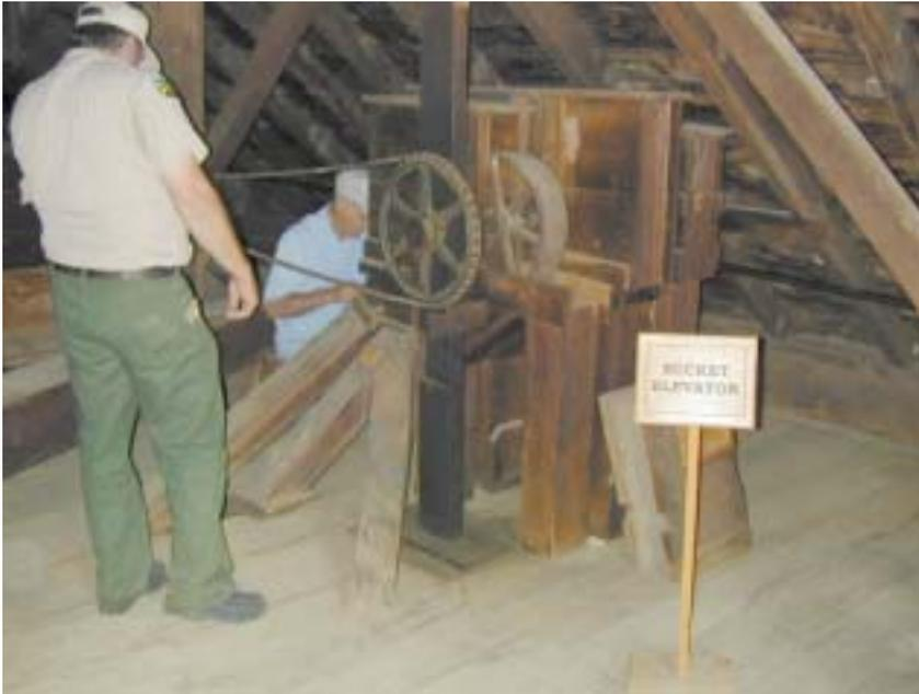
At left are the heads of just three of the many bucket elevators in the mill. From the elevators a complex system of chutes (trunks) lead to various bins and machines. By setting the gates in the chutes the flow chart of the mill could be changed as suited the milling work to be done.
