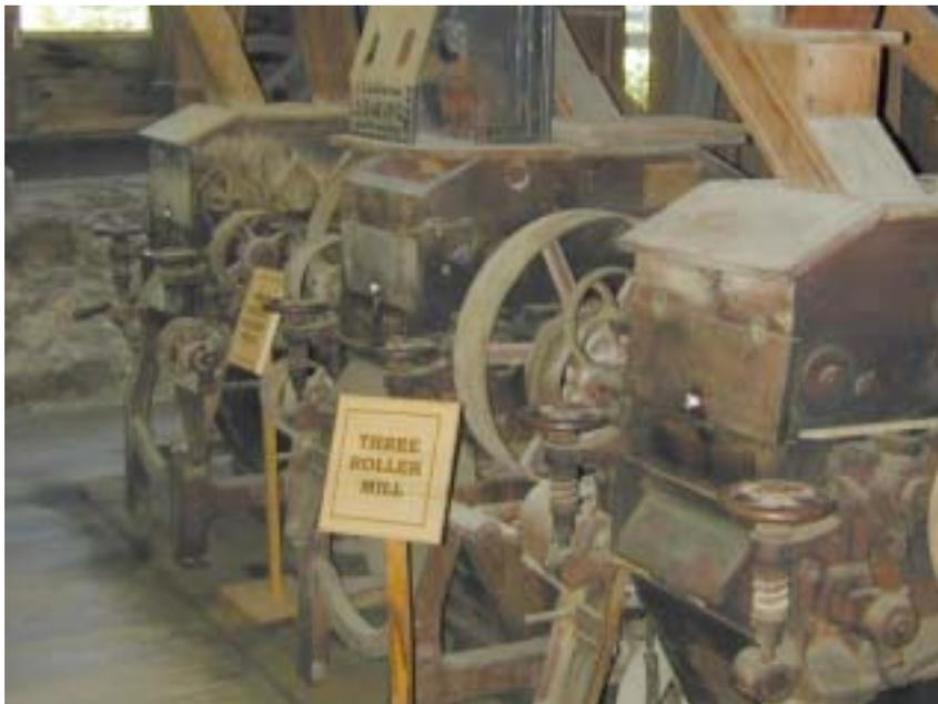
***The three flour milling roller mills. Each machine has two separate mills in it. They are driven by a line shaft in the basement below them.***
